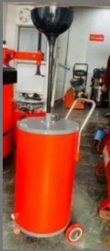
waste oil drain
